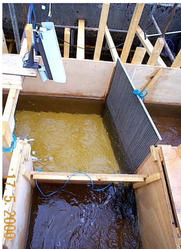
**Plate 3.3 Experimental apparatus used in bar rack trials at Gaur (Clough *et al.* 2000).**
