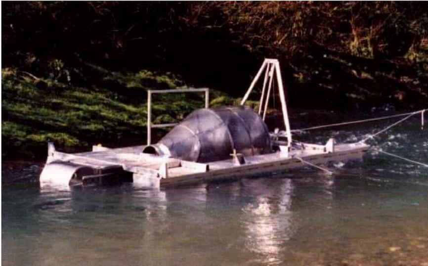
**Plate 7.2 A rotary screw trap. Flow rotates the barrel and fish present in the flow are lifted into a holding chamber. The trap takes a small sample of the total channel flow.**
