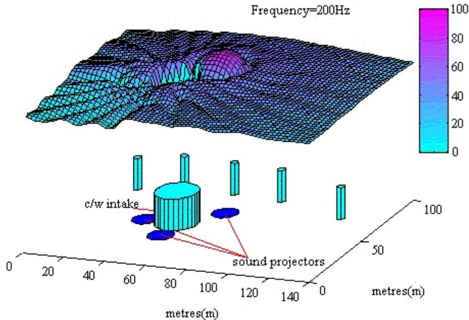
**Figure 3.17 PrISM acoustic model of the acoustic deterrent field at Doel nuclear power station, Belgium (Subacoustech Ltd).**
