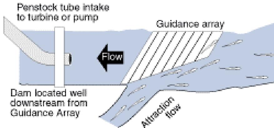
**Figure 3.13 Diagram of the GFFB™ in use as a downstream guidance system ([www.smith-root.com](http://www.smith-root.com)). Note that fish often turn to face the flow when confronted with a barrier.**
