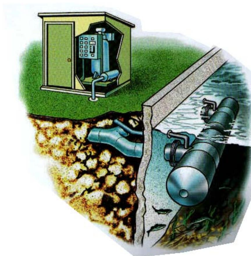
**Figure 3.8** Illustration of bulkhead mounted PWWC screen array with manifold and air backwash system; the compressor is located in a bankside hut but could be located in any neighbouring building. (courtesy Johnson Screens)
