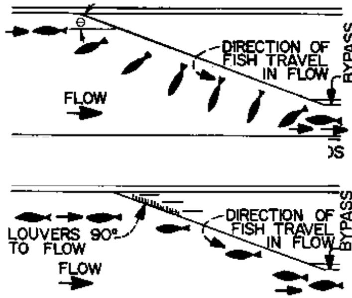
**Figure 5.4** Fish movement in front of angled screens and louvres. Lower diagram applies when the channel velocity is below or near the maximum sustainable swimming speed of the fish, upper diagram when channel velocity exceeds the swimming speed of the fish (Rainey, 1985).
