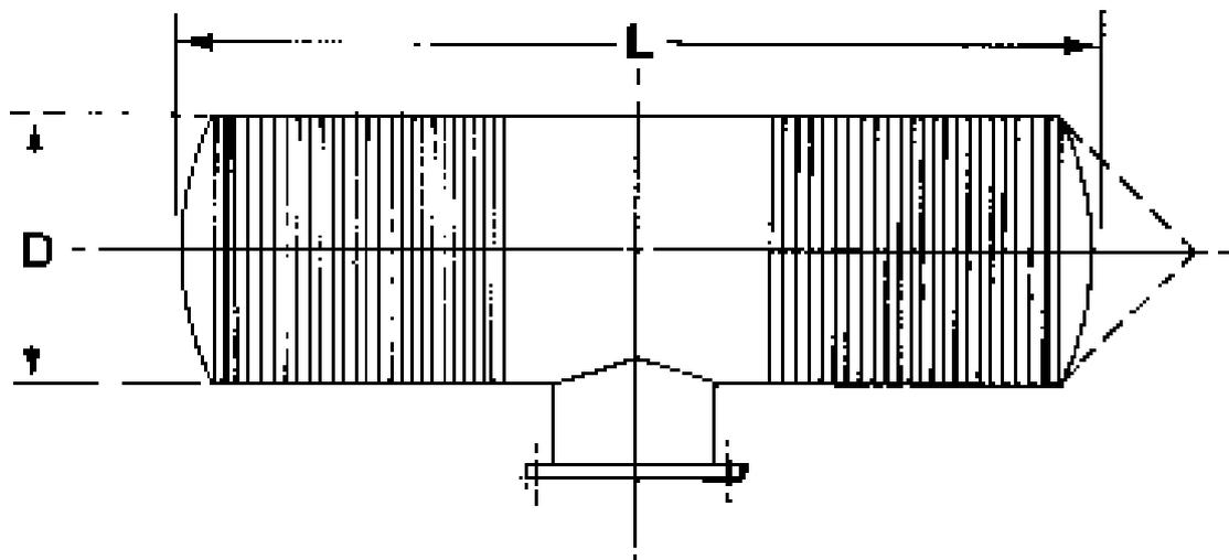
**Figure 3.5 The basic form of the Passive Wedge-Wire Cylinder (PWWC) Tee-Screen (courtesy Johnson Screens)**
