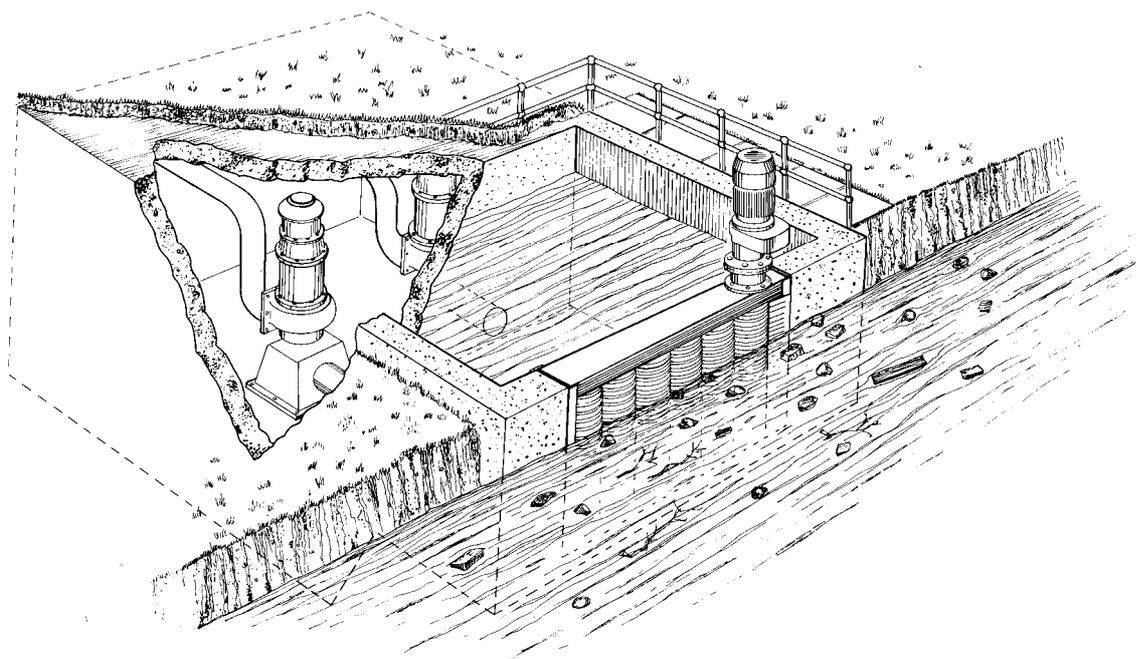
**Figure 3.2 Schematic of Rotary Disc Screen**
