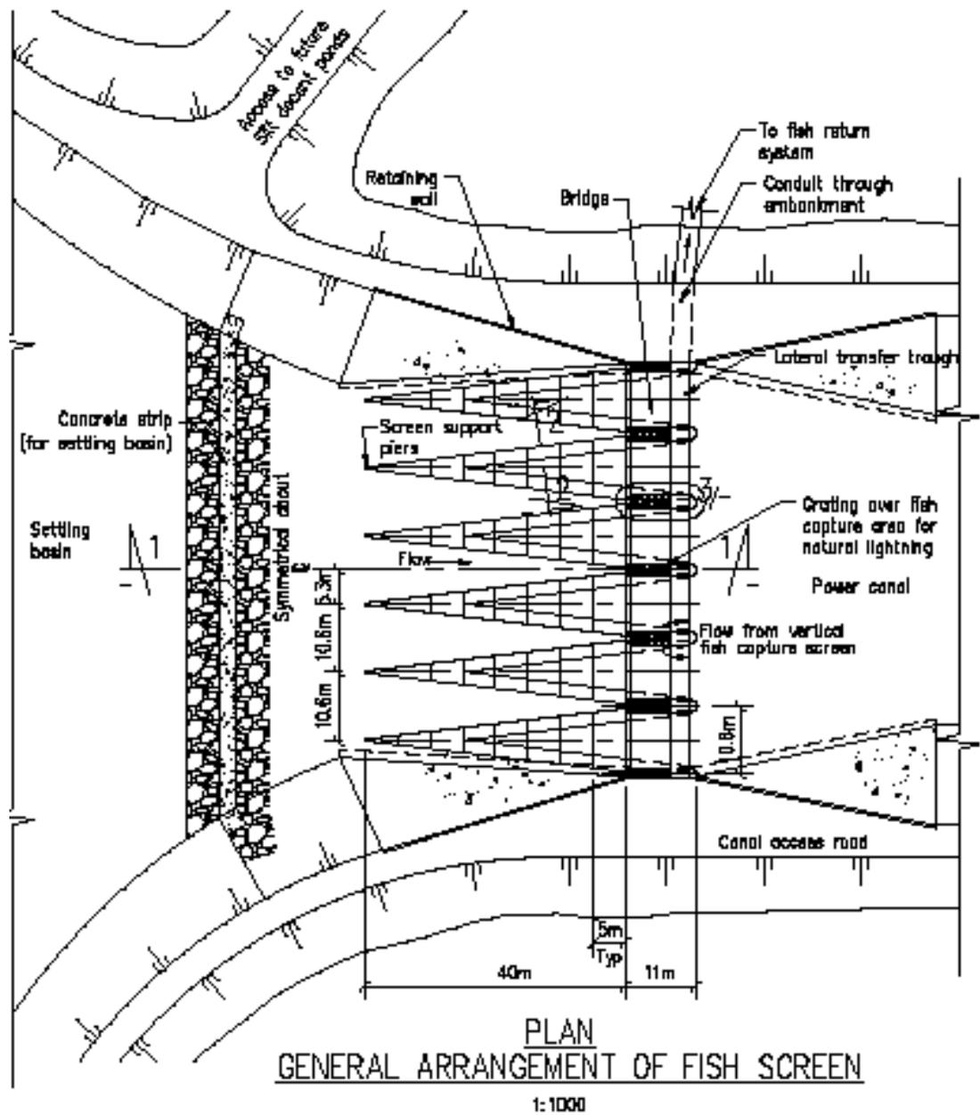
**Figure 3.11 River Waitiki arrangement plan for the Labyrinth screen**
