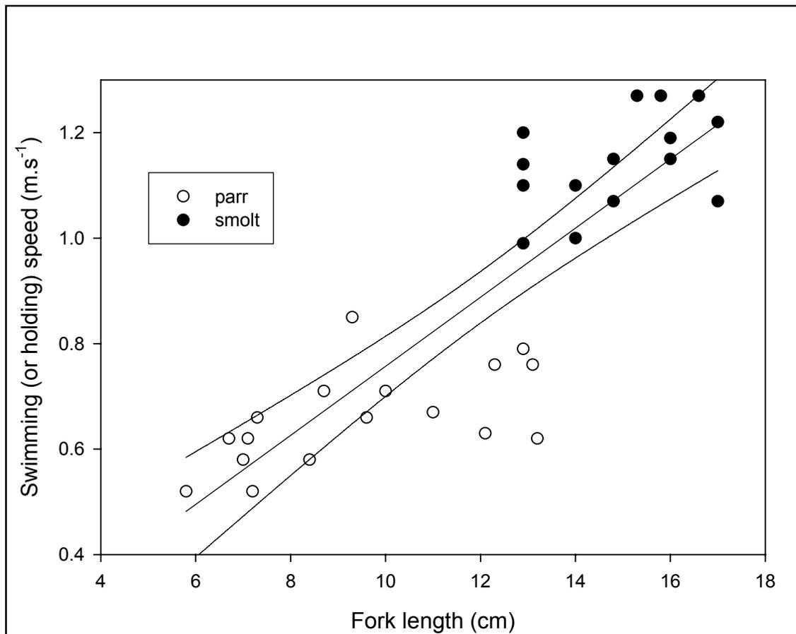
**Figure 5.1** The relationship between fork length and swimming speed maintainable for at least 200 min for Atlantic salmon parr and smolts. Dotted lines are 95% confidence intervals (after Peake & McKinley, 1998).
