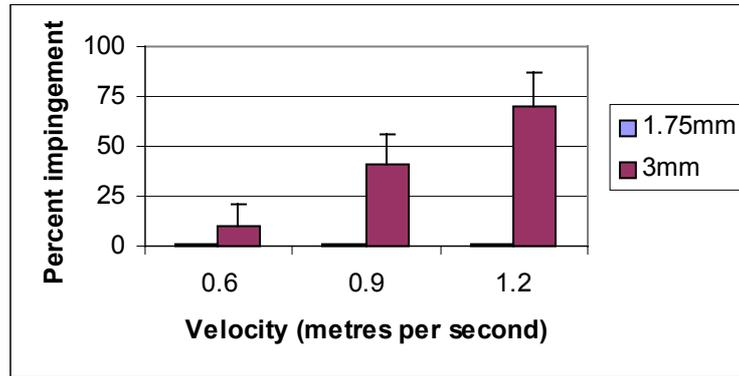
**Figure 5.3 Impingement of Pacific lamprey juveniles on a wedge-wire screens with different spacings over a range of approach velocities (after Moursund *et al.*, 2003).**
