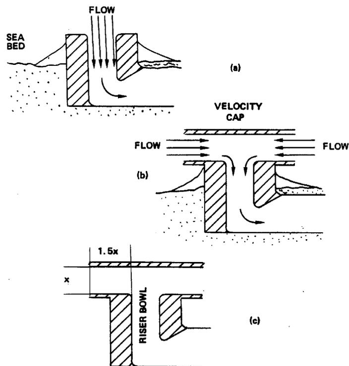
**Figure 3.19 The velocity cap: (a) section of uncapped intake showing vertical draw-down pattern, (b) section of capped intake showing horizontal flow pattern, (c) as (b) but showing critical relationship between vertical opening [x] and length of horizontal entrance [1.5x] for fish reactions (after Schuler and Larson, 1975).**
