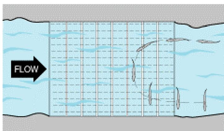
**Figure 3.21 Diagram showing fish movement in response to the GFFB electric fish barrier. In the diagram, the energisation voltage of the electrode strips increases from right to left of the diagram. The fish turn away at a point depending on their length and hence the voltage received along the body ([www.smith-root.com](http://www.smith-root.com)).**
